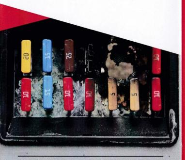
Damage to the circuit protective device when a non-standard fuse was used
