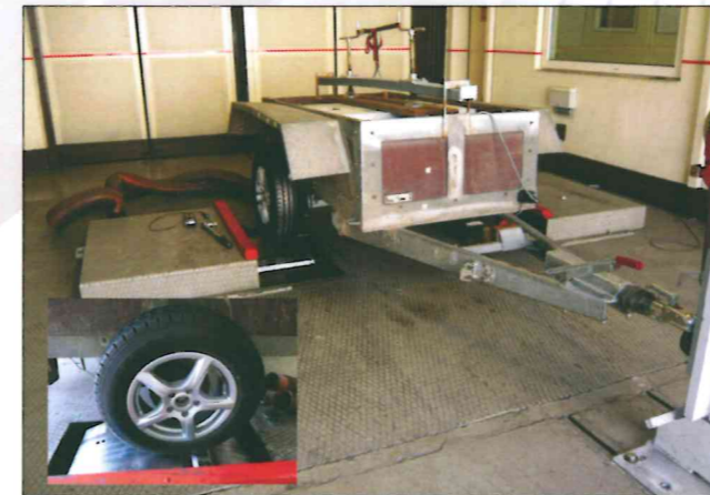
Fig 6 (above) shows the test rig at AL-KO Kotz in Germany where a rigorous test programme was positively conducted on various steel and alloy wheels all fitted with the new WSL Caravan Wheel Safety Bolt. The test was conducted in an overload scenario at high temperatures to achieve a significant safety margin.
